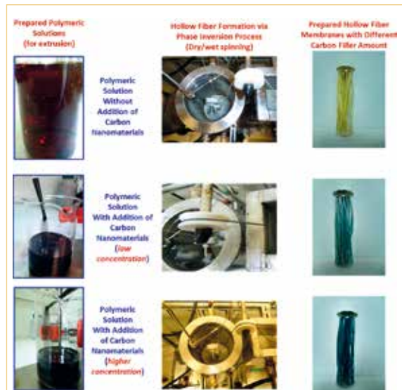
Characteristic images depicted the total process of hollow fiber membranes fabrication (initial solution to final product)
