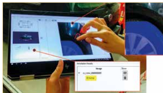
The user can visualize the results, inspect the surface and annotate damages using a portable solution or a cloud interface
