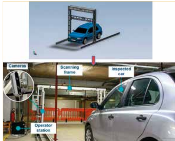
The INVIVO system comprises multiple cameras, lighting and a scanning frame.
