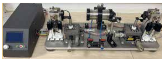
The optical / optoelectronic unit of the prototype consisting of the two lasers properly mounted and temp. stabilized and the gas cell in between
