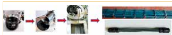
Mixed matrix hollow fiber membranes process steps: from dope solution to developed hollow fibers mounted on a PVC module
