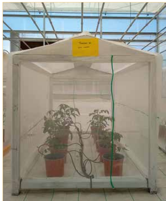
Small-scale greenhouse covered by the SiO 2 coated screen
