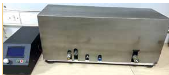
The prototype consisting of the optical / optoelectronic unit and the control and data acquisition system on the left
